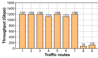
Figure 16: Throughput of different traffic routes (512B packets). In real deployment, we prefer (3) for stability and ease of maintenance. For table size, we borrow the horizontal table splitting technique from Sailfish [41] to share large tables among more gateways.
