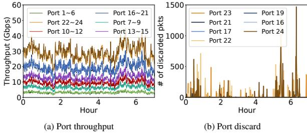
**Figure 3: Load imbalance among equivalent upstream links of an Aggregation switch in production data center.**
