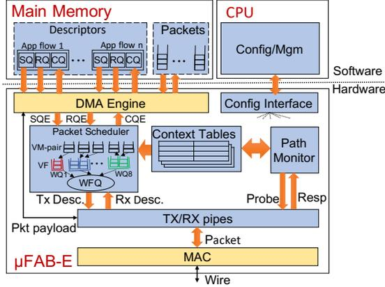
Figure 8:  $\mu$ FAB-E on FPGA-based SmartNIC.
