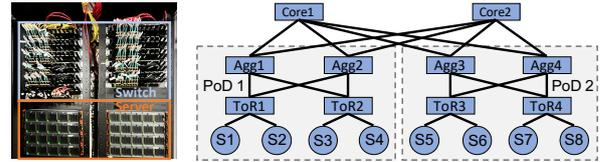
Figure 10: Testbed topology.
