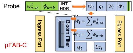
Figure 9:  $\mu$ FAB-C on P4 programmable switch.
