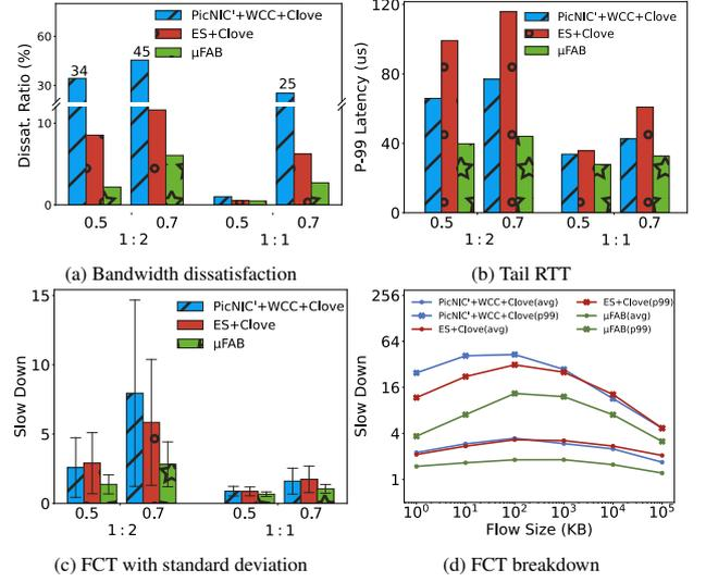
Figure 17: Performance under real workload with 1:2, 1:1 over-subscription network and loads of 0.5 and 0.7.
