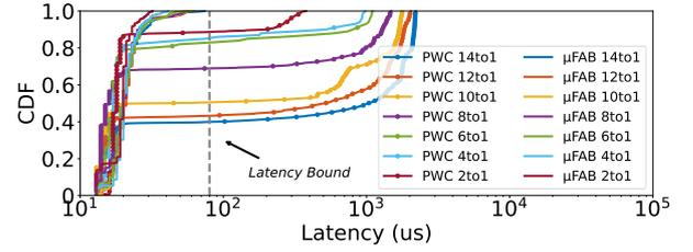
**Figure 4: RTT under various incast degrees.  $\mu$ FAB can bound tail latency as the incast degree increases, while the tail latency of PicNIC'+WCC+Clove (PWC) increases. (Case-1)**
